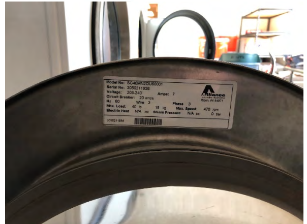
SECTION 3.5: BOTH COMMERCIAL WASHERS IN THE LAUNDRY ROOM ARE CURRENTLY UNDERSIZED AT 40 LB CAPACITY.
