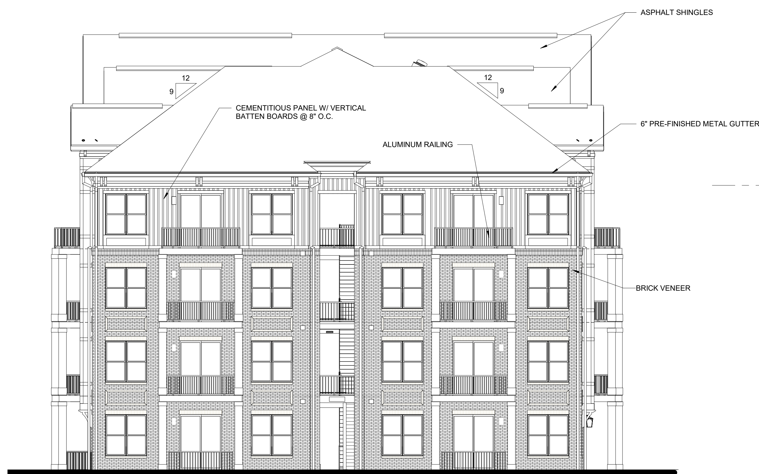
1 BLDG TYPE II - LEFT ELEVATION 1/8" = 1'-0"
