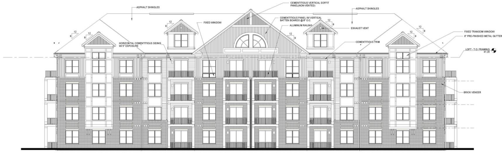
2 BLDG TYPE II - REAR ELEVATION 1/8" = 1'-0"
