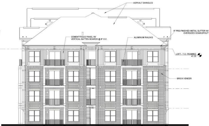
2 BLDG TYPE I - RIGHT ELEVATION 1/8" = 1'-0"
