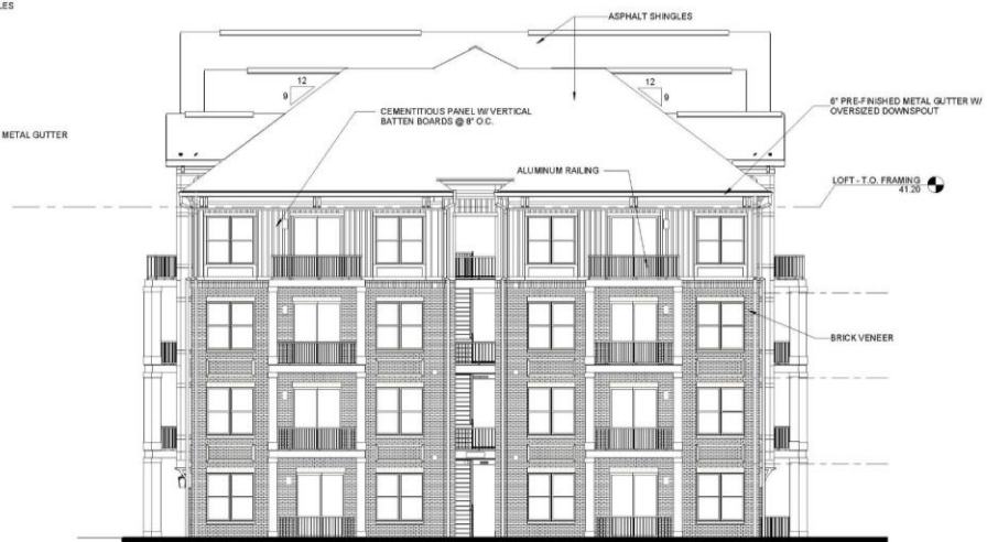
2 BLDG TYPE II - RIGHT ELEVATION 1/8" = 1'-0"
