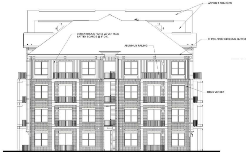
1 BLDG TYPE II - LEFT ELEVATION 1/8" = 1'-0"
